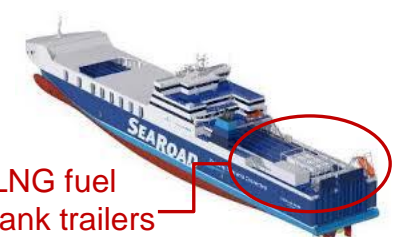
SeaRoad, RoRo ferry, mobile LNG tanks, exchanged via trailers
